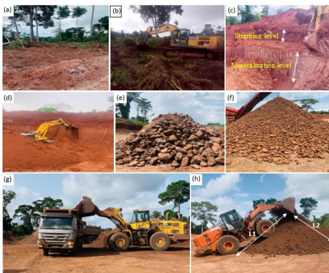
Fig. 8. Field photographs of activity. a, b: Clearing using a hydraulic shovel; c: Stripping with shovel; d: Photography showing manganese ore mining; e, f: Heap of screened manganese ore of different grain sizes; g: Loading and transporting manganese ore; h: Manganese ore destocking L1: first measured length; L2: second measured length
