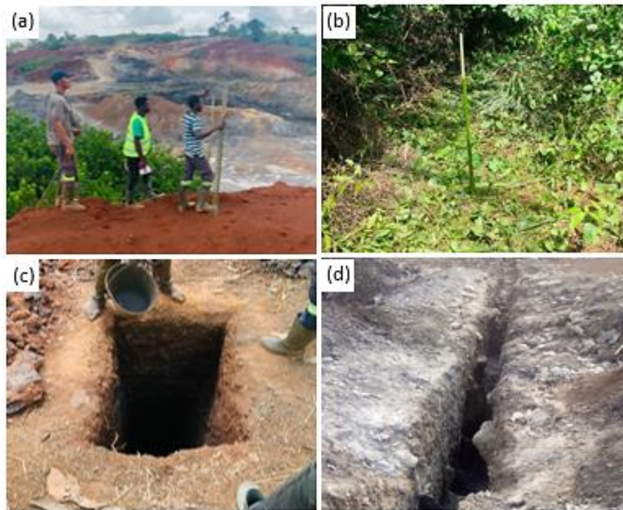
Fig. 7. Layering work. staking (a), Cleared area (b), Well (c) and trench (d) made during prospecting work
