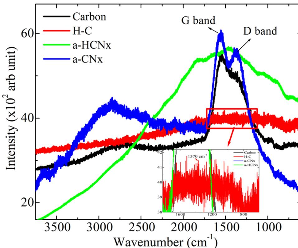
Figure 5. Raman spectra of carbon, a-HC, a-HCN and a-CN film deposited by different plasma deposition methods.
