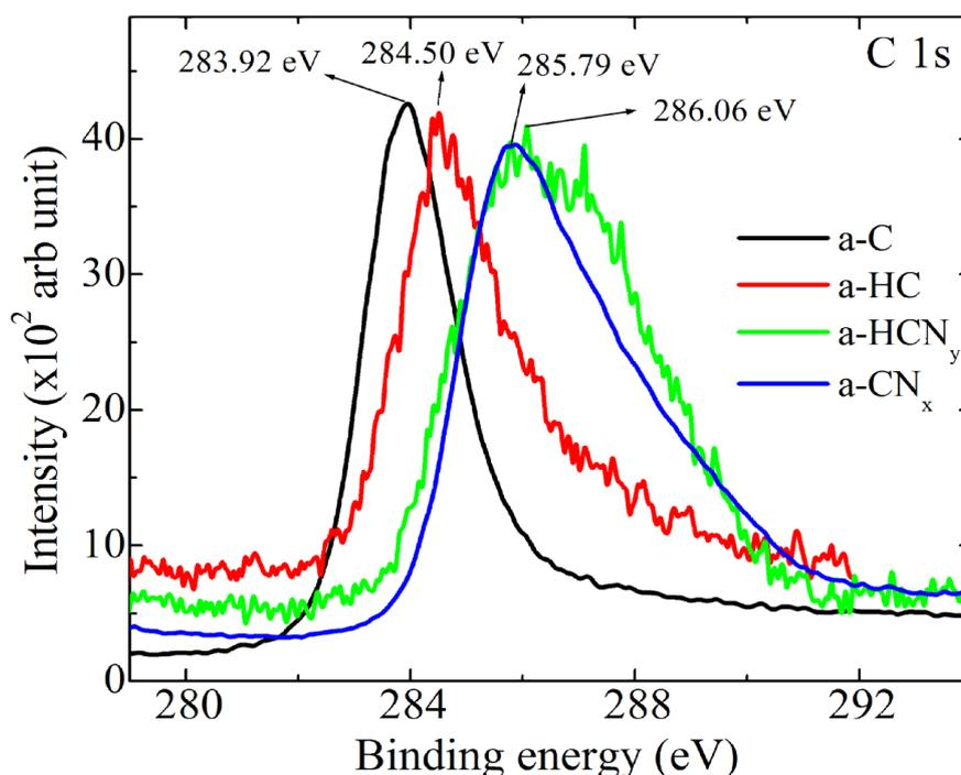
Figure 2. Typical C 1s XPS spectrum of a-C, a-HC, a-CN<sub>x</sub> and a-HCN<sub>y</sub> films. The intensity scales for the C spectra are not the same.
