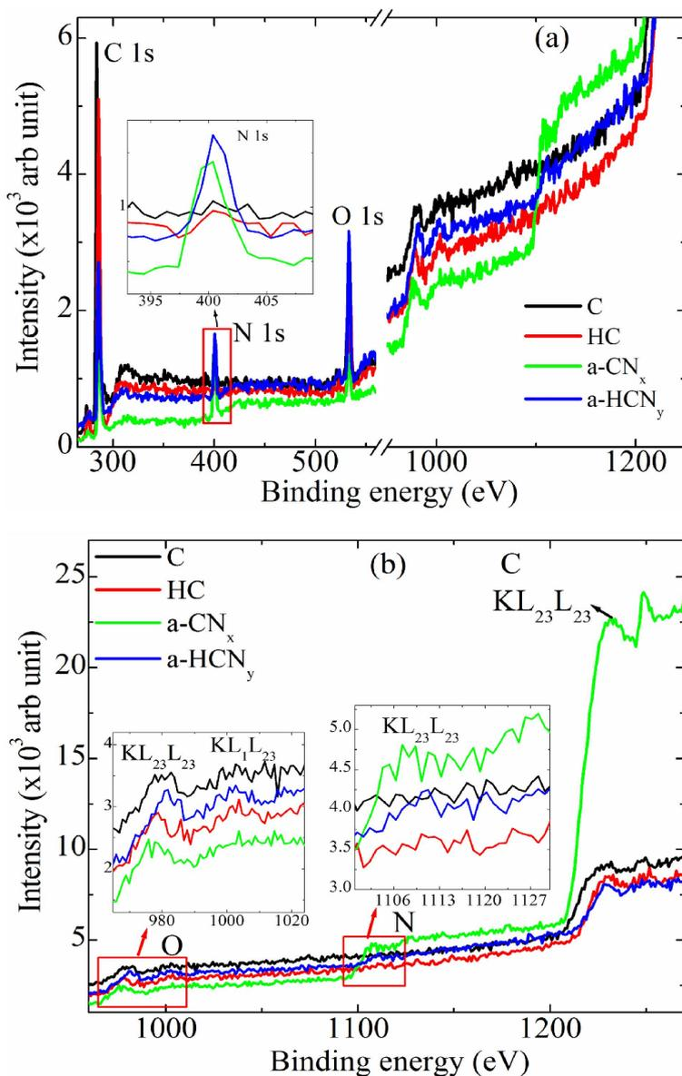
Figure 1. (a) Full scale (260 eV to 1250 eV, with a break at 560 eV to 950 eV) XPS spectrum of a-C, a-HC, a-CN<sub>x</sub> and a-HCN<sub>y</sub> films. In the inset of figure (a), the zoomed area of N 1s peak intensity is illustrated. (b) Auger lines (951 eV to 1270 eV) of the corresponding films and in the inset the zoomed area of O (KL<sub>23</sub>L<sub>23</sub>, KL<sub>1</sub>L<sub>23</sub>) and N (KL<sub>23</sub>L<sub>23</sub>) Auger lines are illustrated. The
