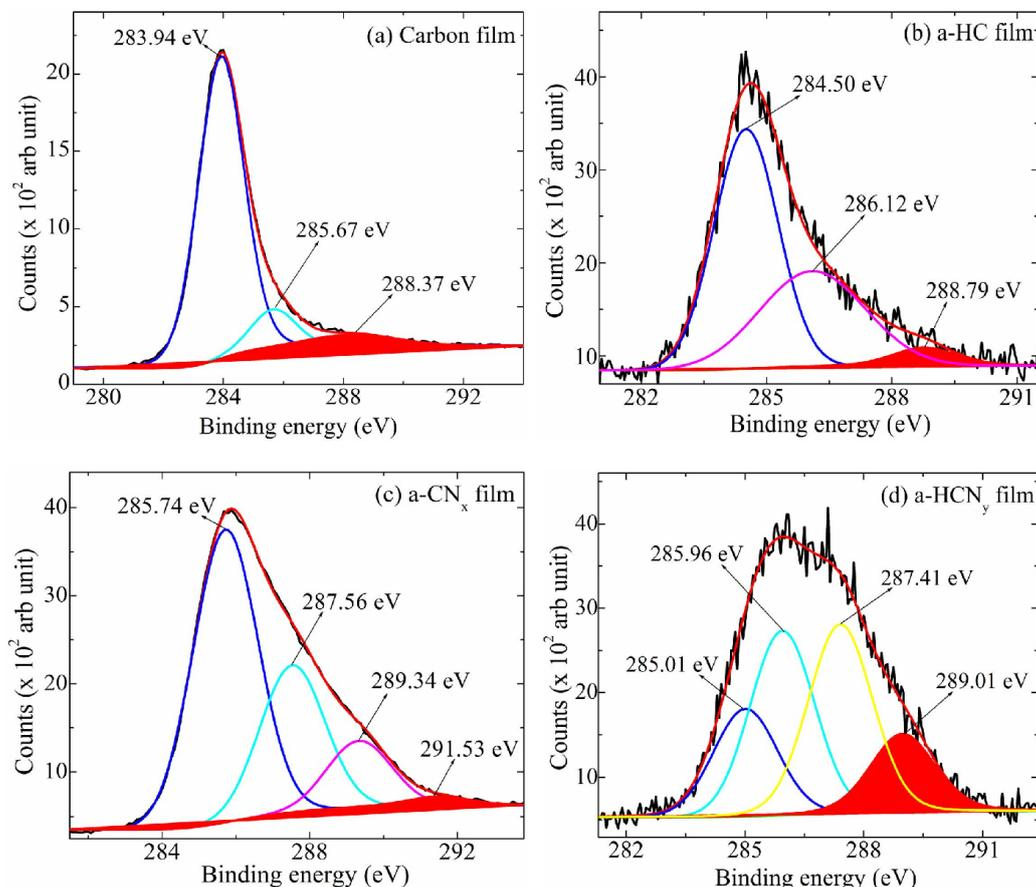
Figure 3. Deconvoluted C 1s XPS spectra of (a) a-C, (b) a-HC, (c) a-CN<sub>x</sub> and (d) a-HCN<sub>y</sub> films. C 1s XPS spectra obtained with Mg *kα* x rays at 23.5 eV pass energy at 0.125 eV/step. The red marked peak area is referred as oxide peak. The data are presented after inelastic background subtraction and using Gaussian fits. The intensity scales for the C spectra are not the same.
