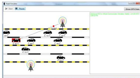
'B' met with an Accident which is shown in Red area. This B Vehicle then communicates with Road Side Unit (RSU). RSU will get all the location information through GPS. RSU then calculates the position of the vehicle by using great circle algorithm and bearing angle.
