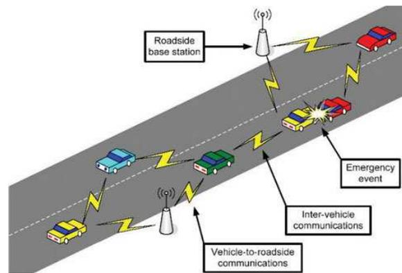
**Fig. 1.1 Communication in VANET (V2V and V2I)**
