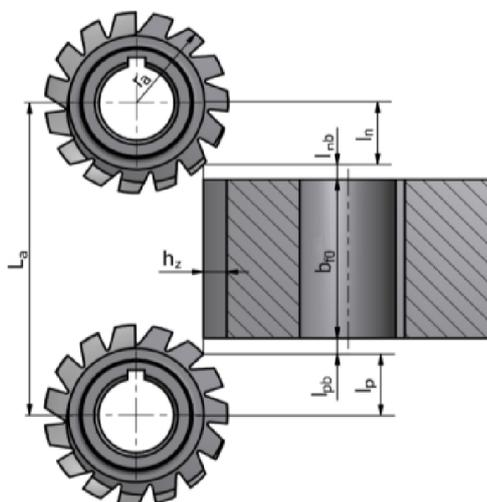
Fig. 7. Slope and run-out of the gear hob
