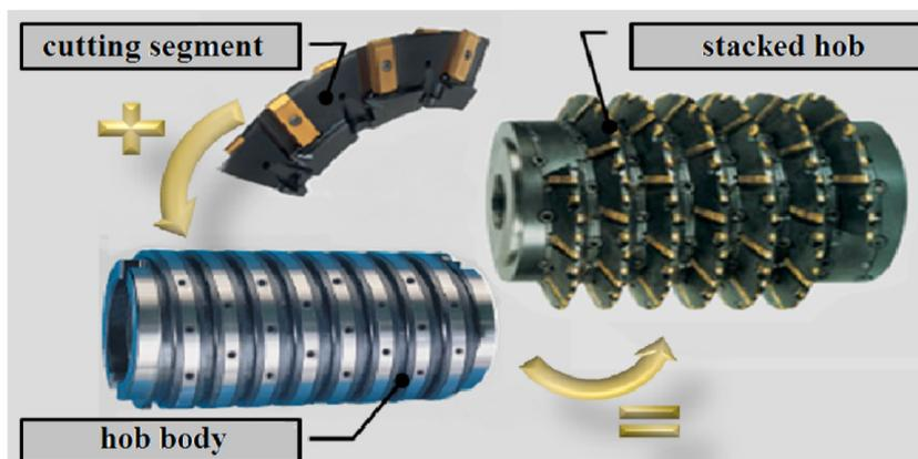
*Fig. 3. Construction of stacked hob*
