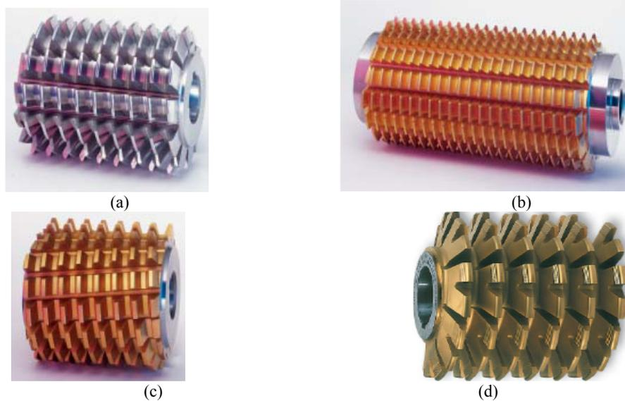
Fig. 1. Selected types of in-feed hobs with solid cutters.
