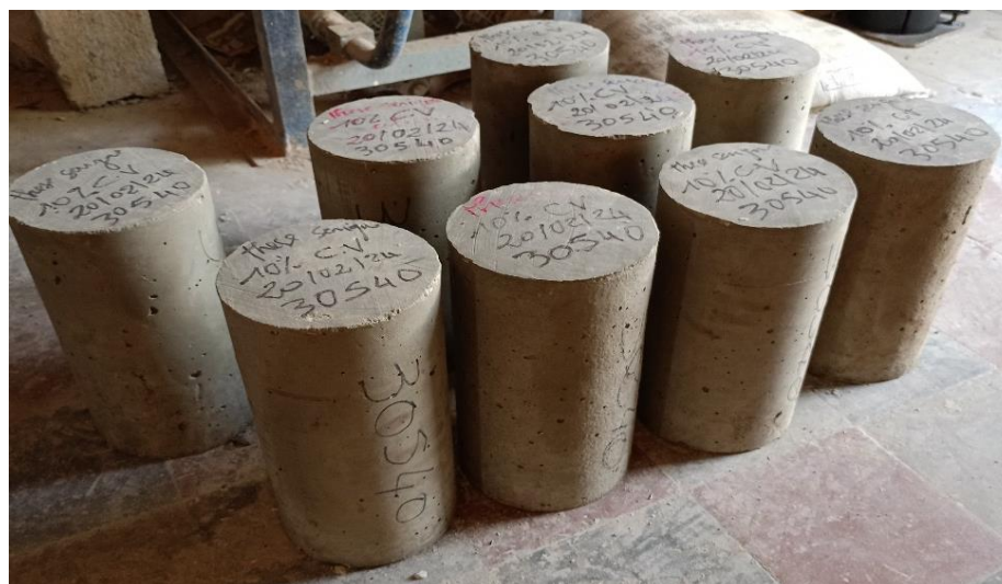
Fig. 3. Improved hydraulic concrete specimens, just after demolding
