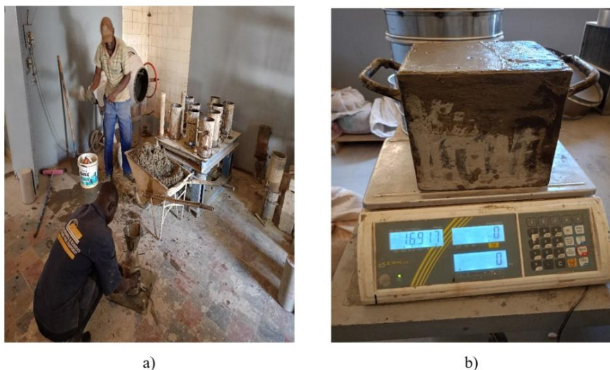
Fig. 2. a) slump measurement and b) measurement of concrete density
