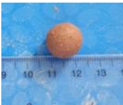
Fig. 1. B catalyst (spherical pellet laterite + kaolinite)
