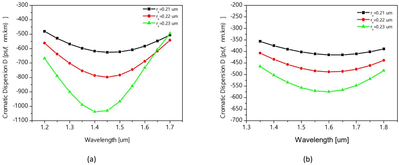
Fig. 4. Chromatic dispersion for (a) X-polarization and (b) Y-polarization
