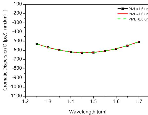
Fig. 2. Dispersion with respect to thickness of PML
