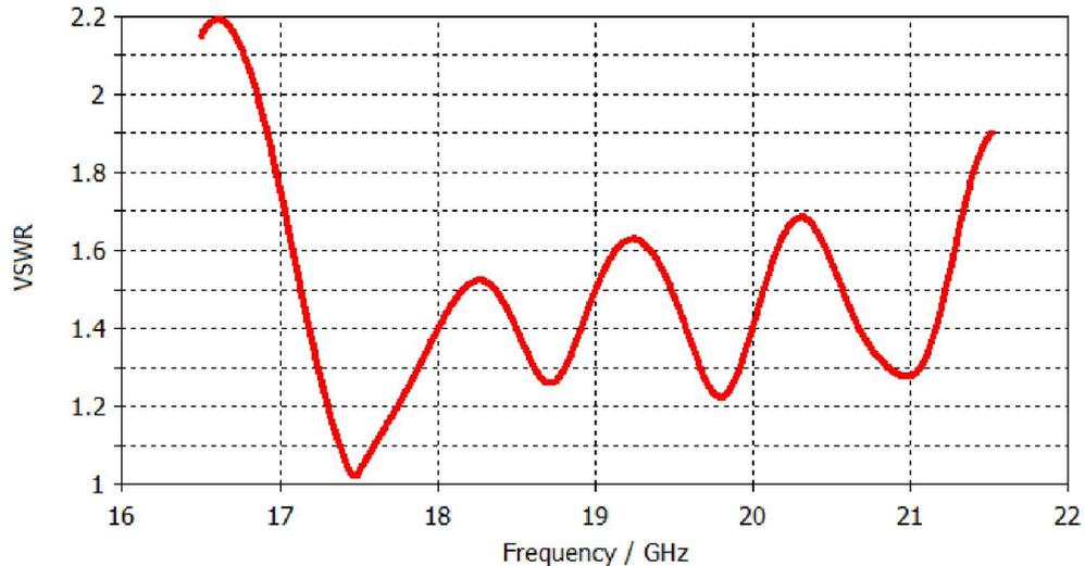
**Fig. 4. Simulated VSWR of the proposed antenna**
