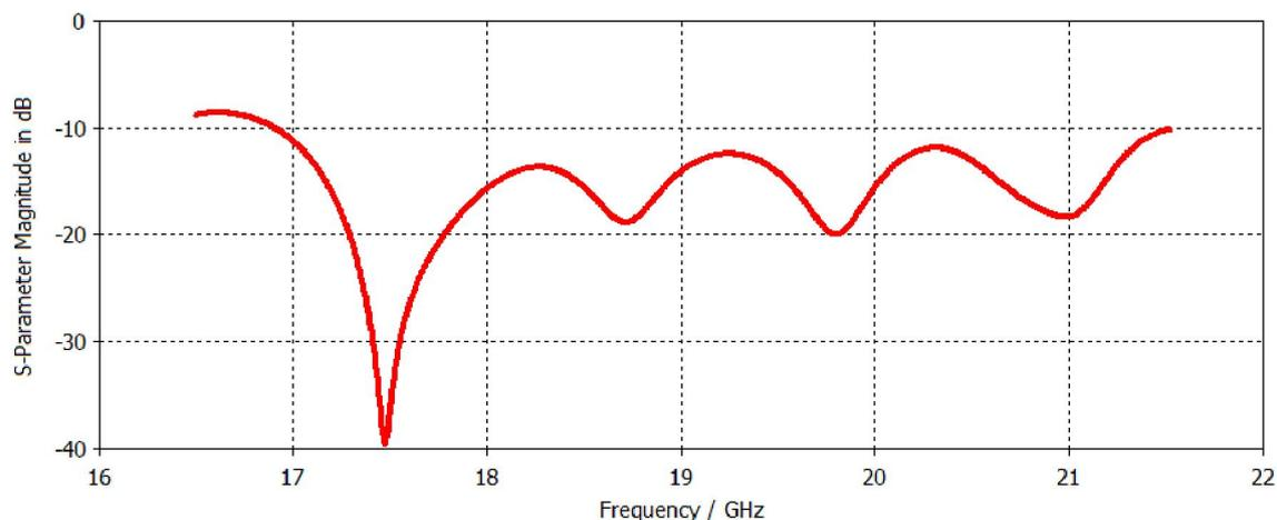
Fig. 2. Reflection coefficient for the cylindrical DRA
