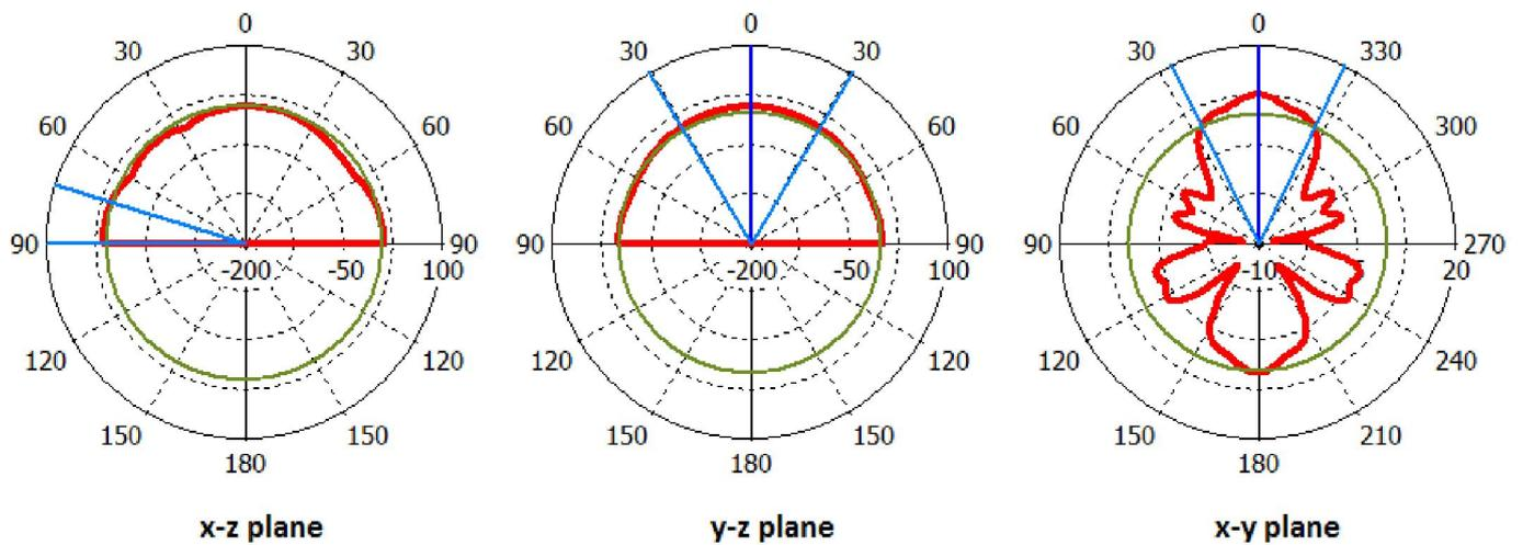
Fig. 7. Simulated radiation patterns of the proposed antenna at 19.8 GHz
