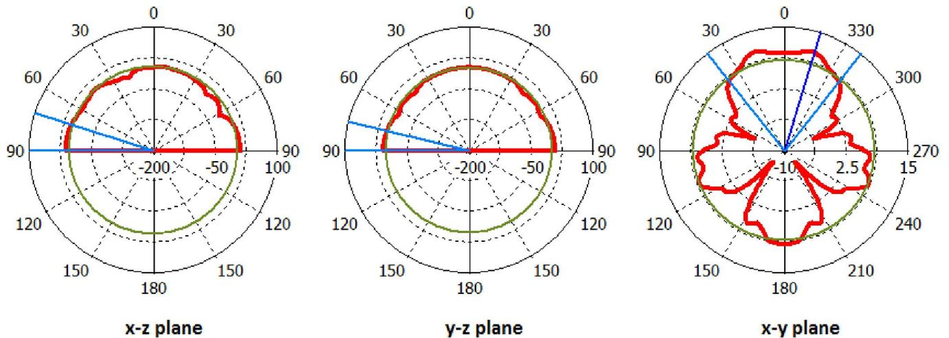
Fig. 8. Simulated radiation patterns of the proposed antenna at 20.986 GHz
