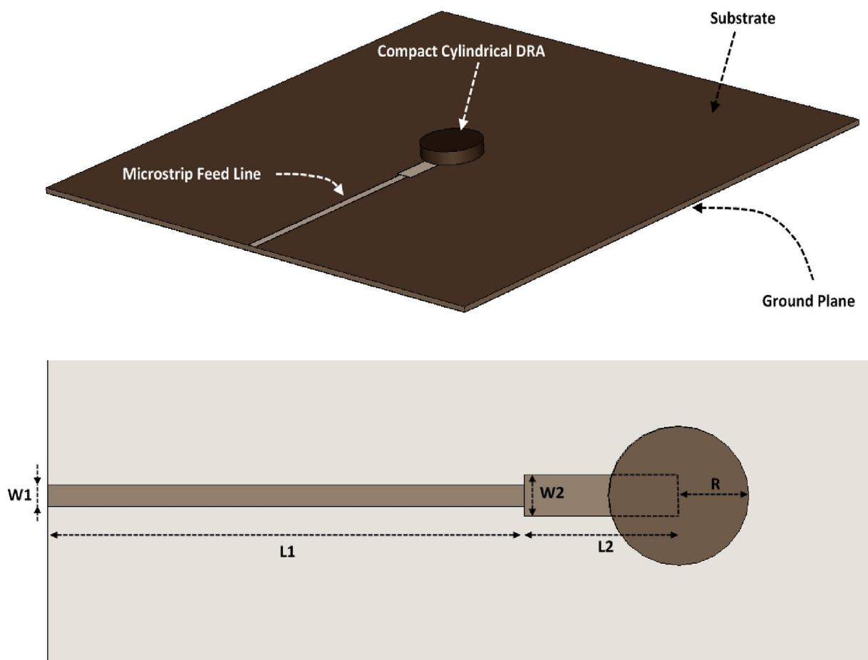
Fig. 1. The geometry of the proposed antenna
