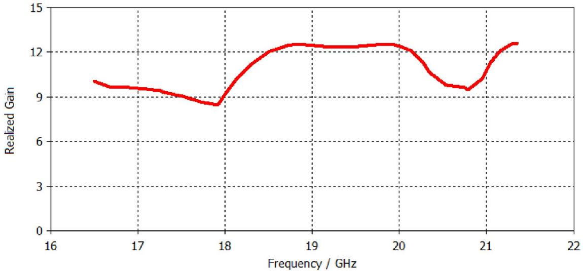
**Fig. 3. Simulated realized gain of the proposed antenna**
