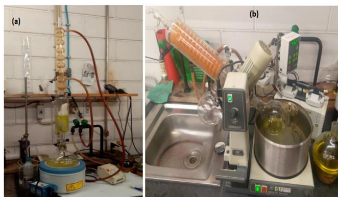
Fig. 3. (a) Soxhlet extraction (b) Solvent evaporation
