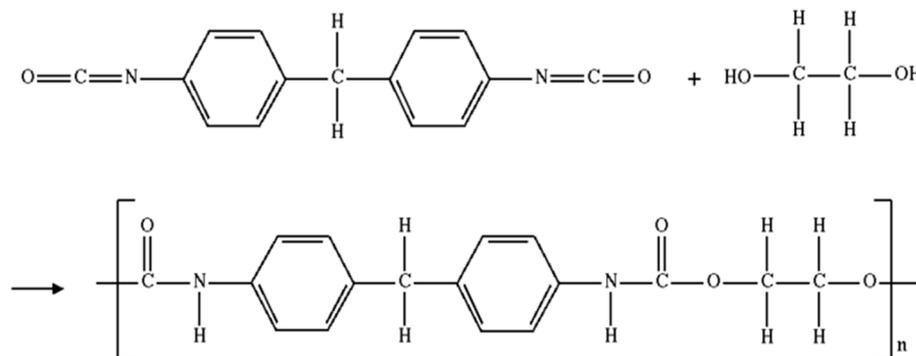
Fig. 4.8 Structure of Polyurethane
