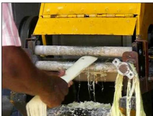
*Fig.3.3 Banana fibre extraction machine*
