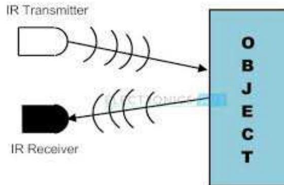
**Figure: 6 Functional Representation of IR Sensor**
