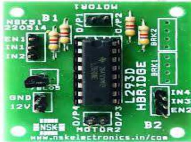
Figure: 10 H Bridge with different ports
