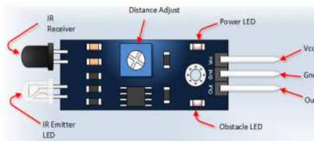
Figure: 5 Functional Pin Diagram of IR Sensor
