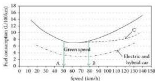
**Fig 1. Relation between fuel consumption and average speed**
