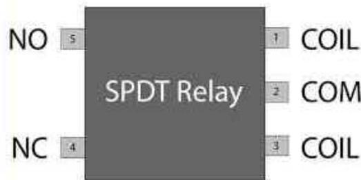
Fig 6. Pin diagram of relay
