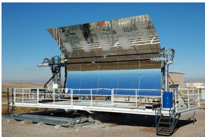
Fig. 3. Sandia experimental collector installed in desert Mojave in South California, 39m 2 adapted from [12]
