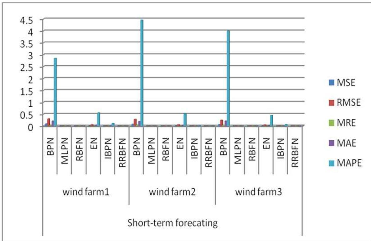
Fig. 17. Comparison of ANN based forecasting models for short-term forecasting
