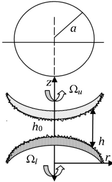
Fig. 1. The geometrical configuration of the bearing system
