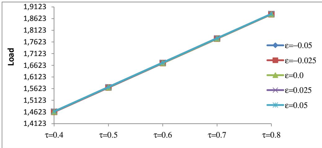
Figure- 7 Variation of Load carrying capacity with respect to  $\tau$  and  $\epsilon$
