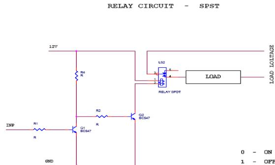
Fig. 3. Relay circuit
