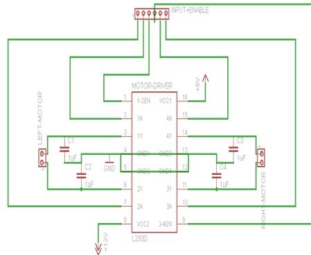
Fig. 5 motor driver chip
