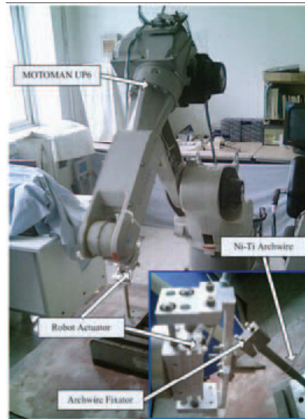
Figure 3: Archwire bending robot based on MOTOMAN UP6
