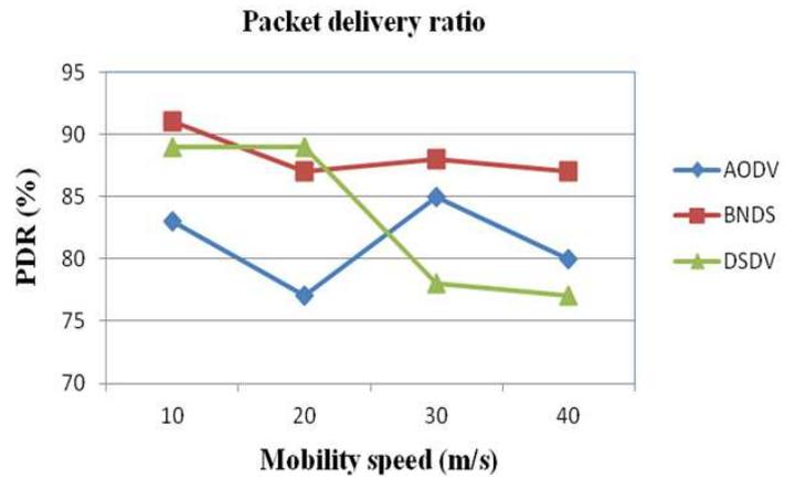
Fig. 4. Mobility speed Vs Packet delivery ratio
