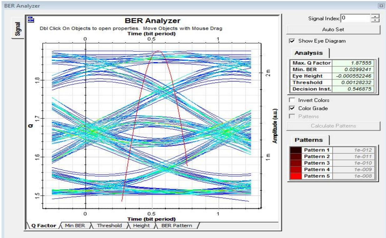
Fig. 2. Eye diagram for 6GHz bandwidth
