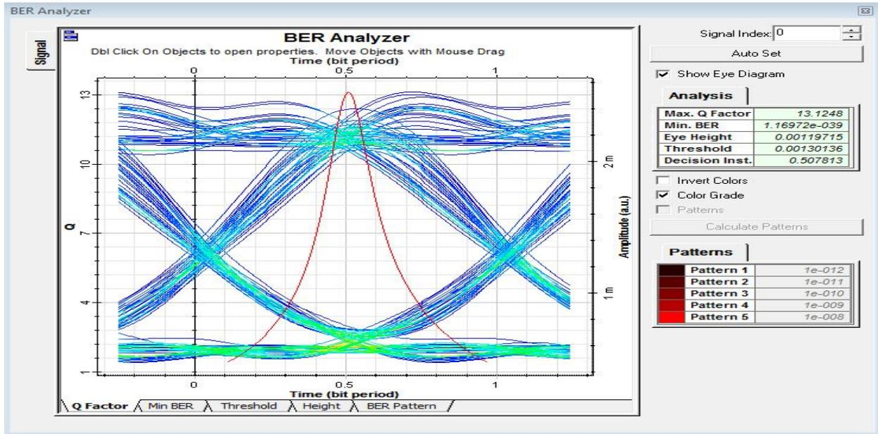
Fig. 6. Eye diagram for 34GHz bandwidth
