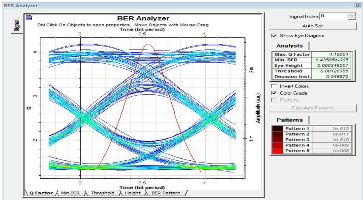
Fig. 3. Eye diagram for 10GHz bandwidth
