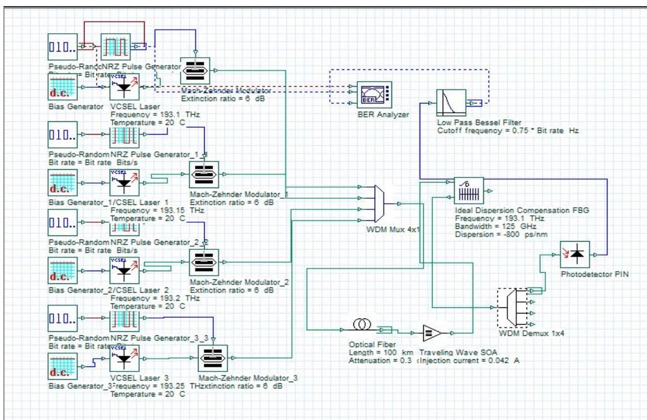
Fig. 1. WDM system using SOA
