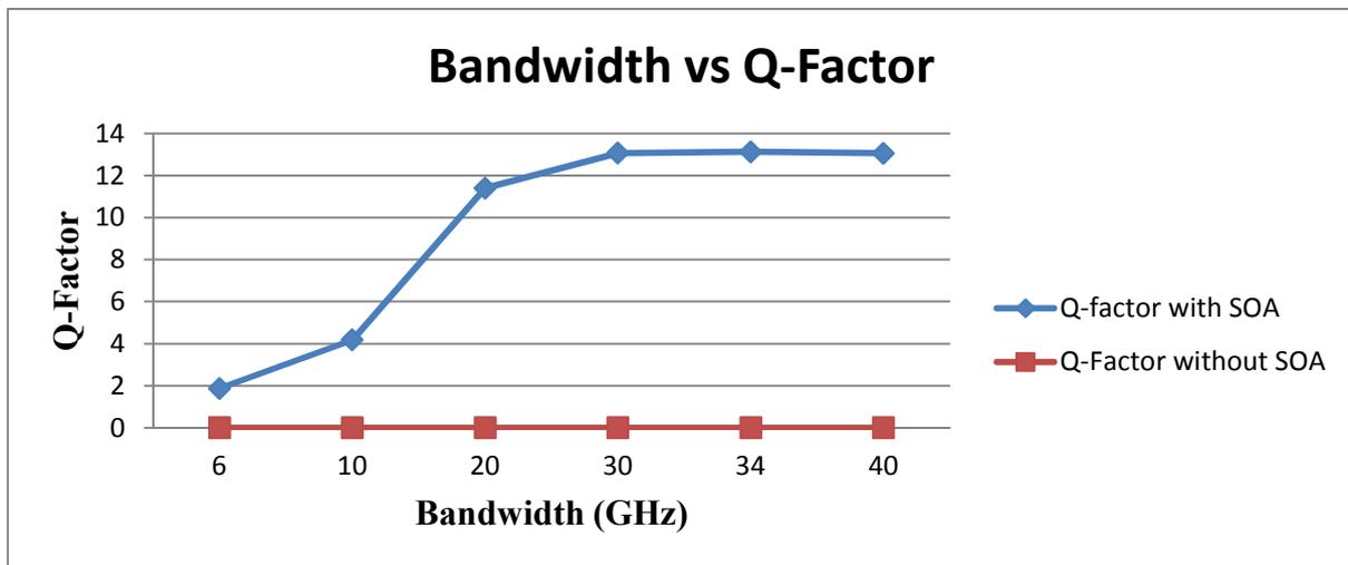
Fig. 10. Plot of Bandwidth vs. Q-factor with and without SOA
