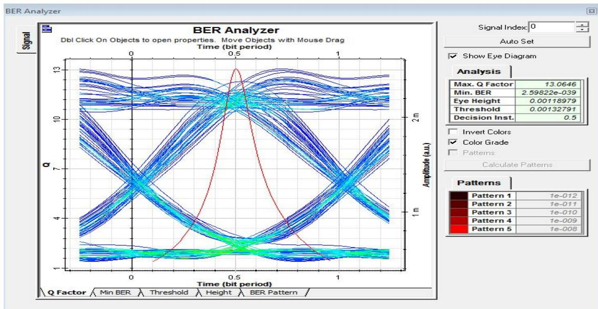
Fig. 5. Eye diagram for 30GHz bandwidth
