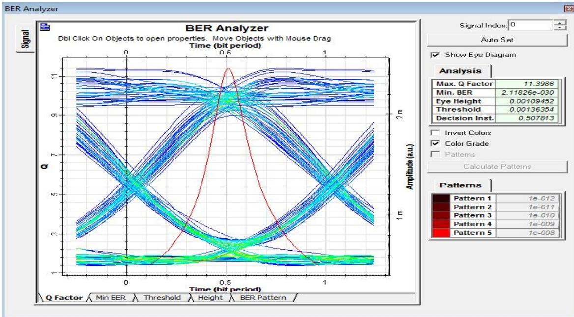
Fig. 4. Eye diagram for 20GHz bandwidth
