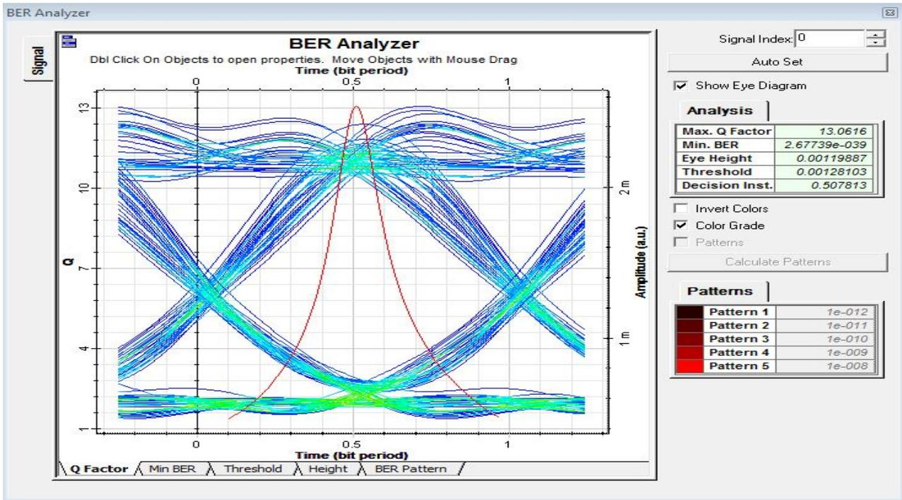
Fig. 7. Eye diagram for 40GHz bandwidth
