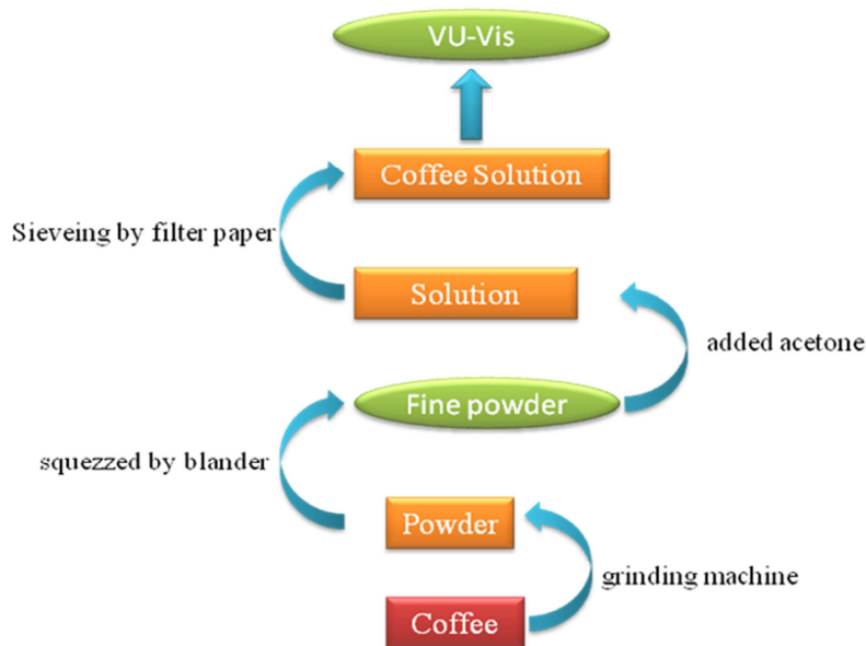
Fig 3 Flow chart of experimental procedure for coffee natural dye-sensitizer
