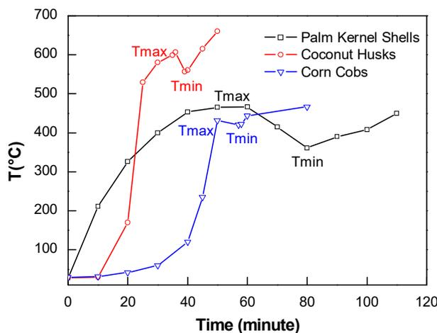
Fig. 2. Temperature measured at the bottom of the biochar stove for the three biomasses.
