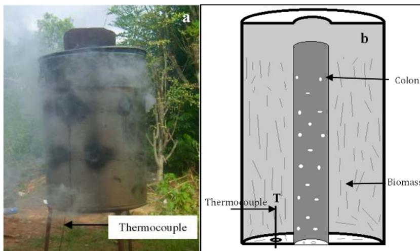
Fig. 1. (a) The photographic image of the biochar stove and (b) its schematic sectional
