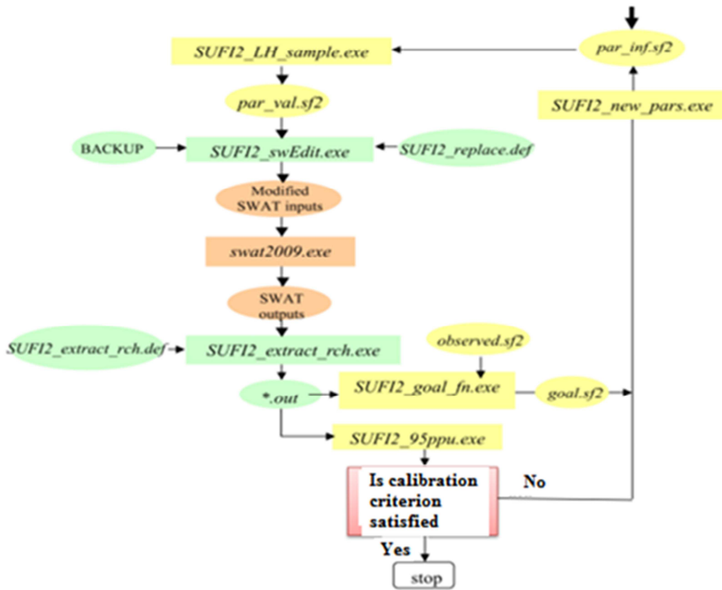
Fig. 6 calibration procedures using the method in the interface SUFI2 SWAT-CUP (Modified Abbaspour, 2011)
